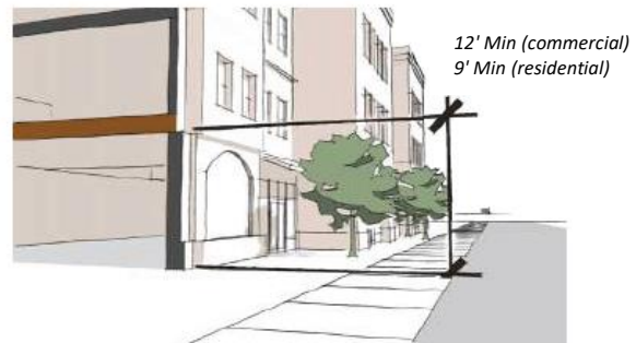
Figure 17.134-14: Ground Floor Plate Height
