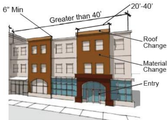
Figure 17.134-11: Building Facade Form Variation
